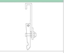
It secure the Jack Bases/U-Heads for lifting.
