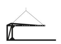
It enables the tableform to lift and fly.
