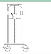
It enables the table form to be adjusted up / down to 1m high and to be moved freely.
