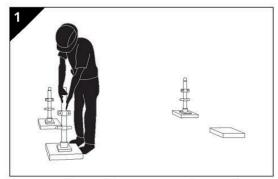
Position the jack base, spaced according to the lengths of the longitudinal and transverse horizontal members.
