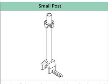
Equipped with a wedge coupler, it is used at the end of the bracket as a guard-rail post, or onto the horizontal members, in order to cut the span of storage or circulation areas.
