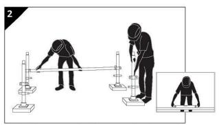
Fit the basic standards or standard into the jack base. Fit the horizontal members. Check the structure is level.
