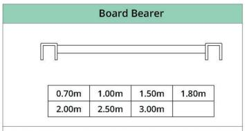
It cuts the span of the boards which constitute the working or access areas.
