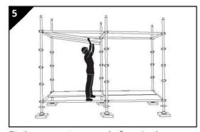
Fit the access trapper platform in the access bay. Lower the ladder. Check continuously that the structure is level.
